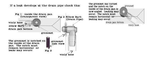
Tip: To prevent the grommet from turning, hold the grommet securely while turning the elbow barb when positioning it to drain.
